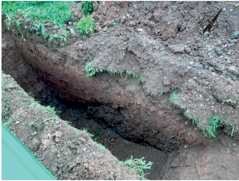
Photograph 6. Pit excavated for percolation testing, showing undisturbed fractured, weathered sedimentary bedrock, overlain by stony red clay and soil.
