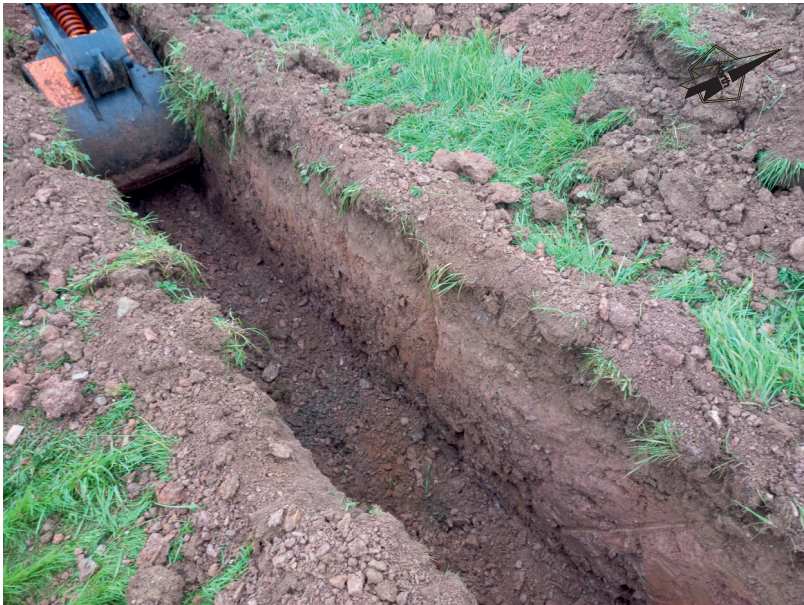
Photograph 3. Detail of horizons of weathered fractured, in-situ, undisturbed, unmineralised sedimentary bedrock, overlain by soils. exposed in Trench 1.
