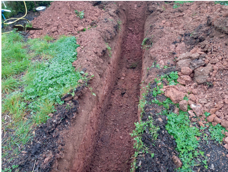
Photograph 5. Detail of intact, undisturbed horizons of soil and stony clays underlain by fractured weathered bedrock in Trench 2.
