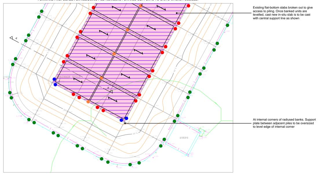
THIS DRAWING IS TO BE READ IN CONJUNCTION WITH DETAIL OPTIONS SK502 / SK503 FOR SPECIALIST CONTRACTOR TO BRING FORWARD PREFERRED OPTION FOR RE-LEVELLING
