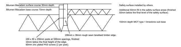
Details of safety surface to be installed by others (not to scale).
