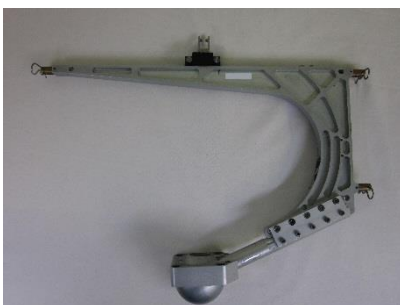
Supporting arm - impact points B, X & R
