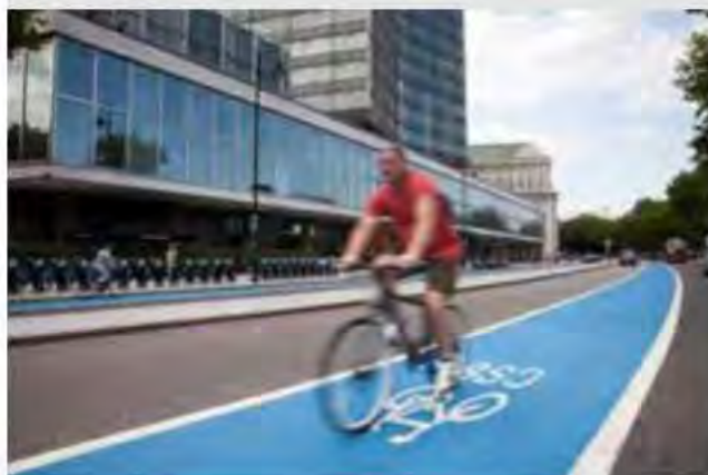
Figure 111: Cycle track demarcated with lines and colour
