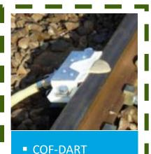
Quantifying the effects of Railhead Treatments on adhesion
