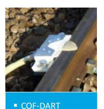
Quantifying the effects of Railhead Treatments on adhesion
