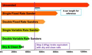
As a result, RSSB is co-funding an implementation project with WMT that seeks pilot these variable sanding configurations in a real railway environment.
