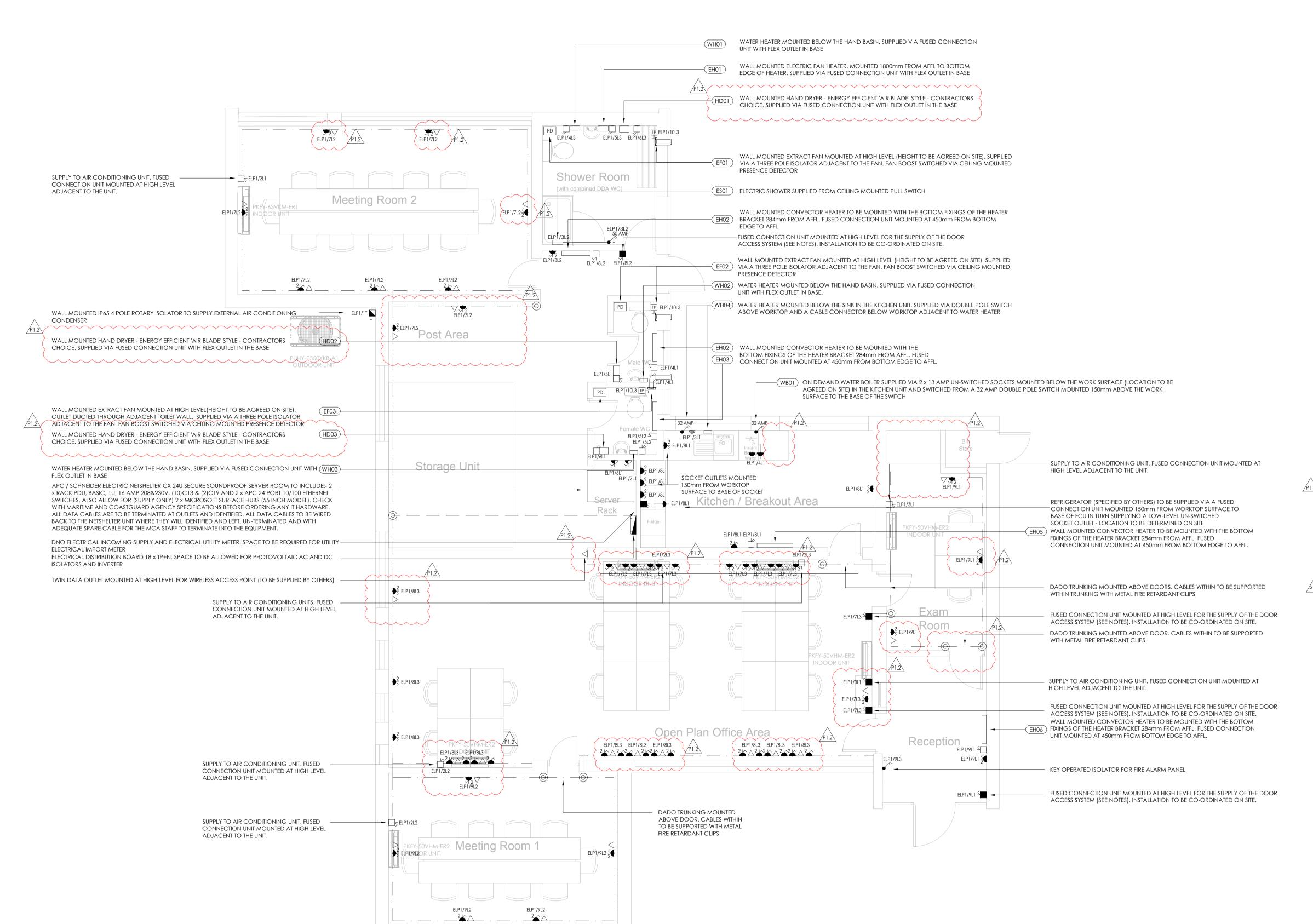
PROPOSED ELECTRICAL POWER AND DATA LAYOUT Scale: 1:50
