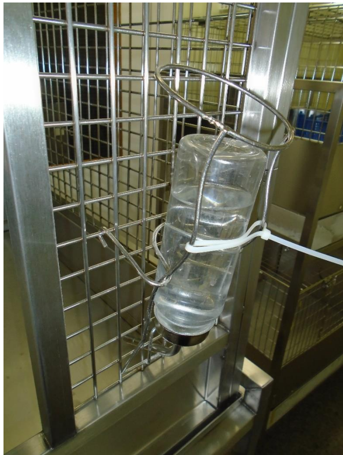
Fig. 9 – The water bottle can be attached to the wire mesh. New water bottle holders would be beneficial. Must be able to hold a 250ml autoclavable bottle. Different sizes could be considered to fit a 500ml bottle also.
