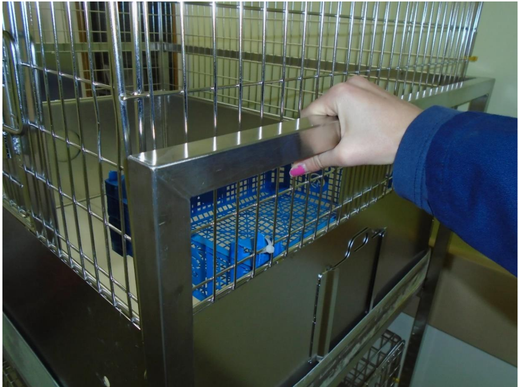
Fig 7. Shows the general height of the external frame. This frame runs across the sides and back to prevent the cages from slipping off. The frame will allow the user to push/pull without the risk of being bitten by the animal inside the cage.
