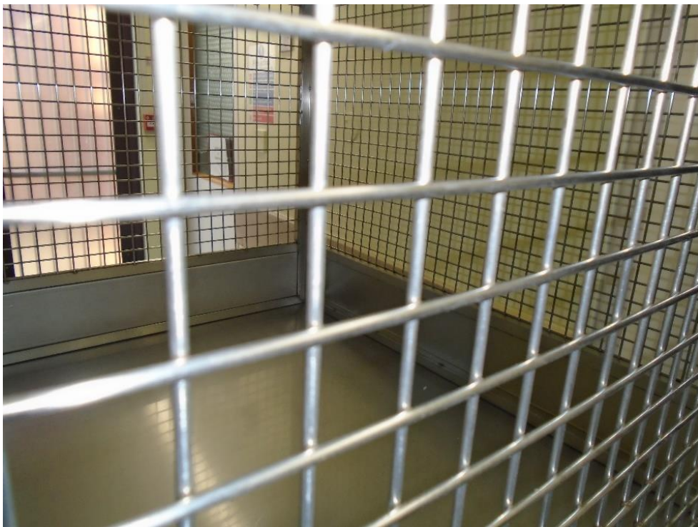
Fig. 11 – Example of the type of wire mesh that is unsuitable for this cage, due to the thickness adding to the overall weight of the cage. It is also not aesthetically pleasing.
