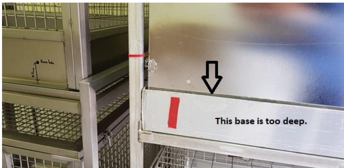
Fig. 13 – The base on the left-hand cage is suitable to hold the panels in place. The base on the right cage however is too deep.
