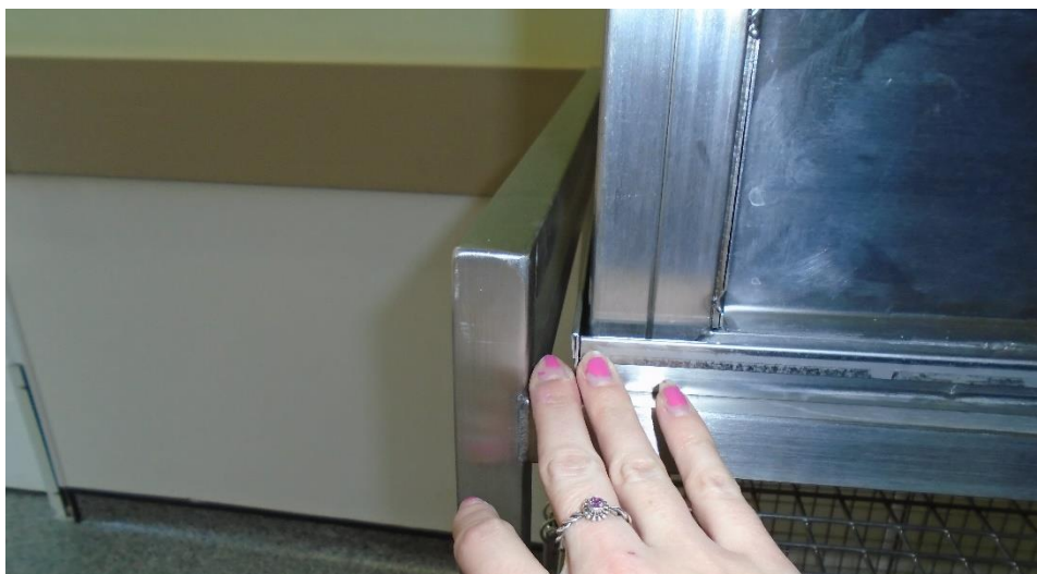
Fig. 12 – The gap between the frame and cage base is too large. Poses a risk of fingers getting trapped. There must be minimal space between.
