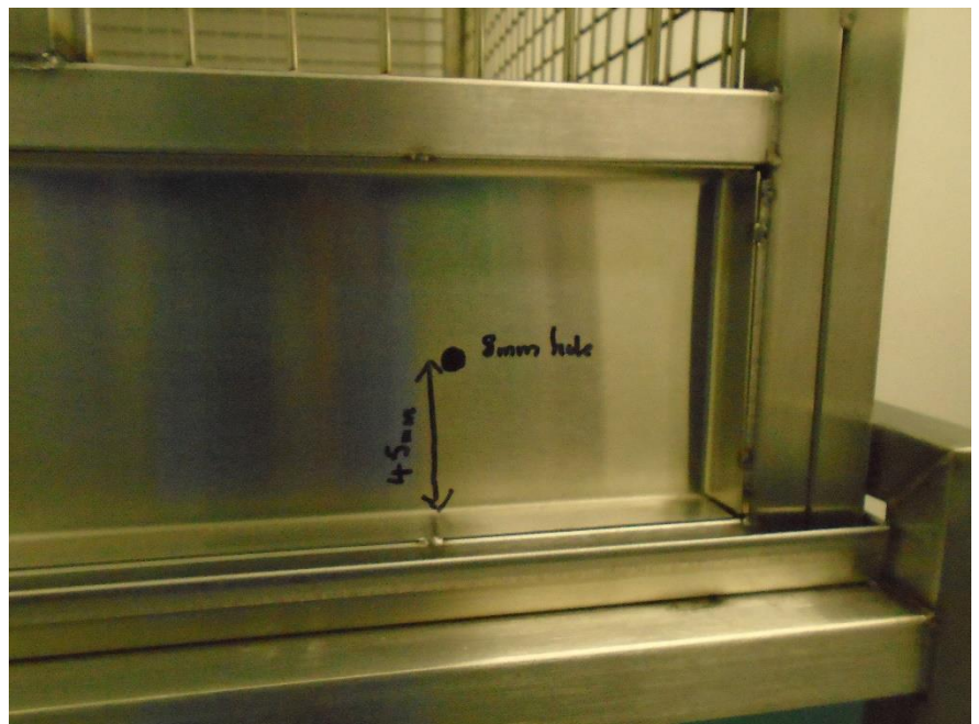
Fig 8. Example of the hole on the solid part of the front panel, allowing a coop cup to be attached to the cage.
