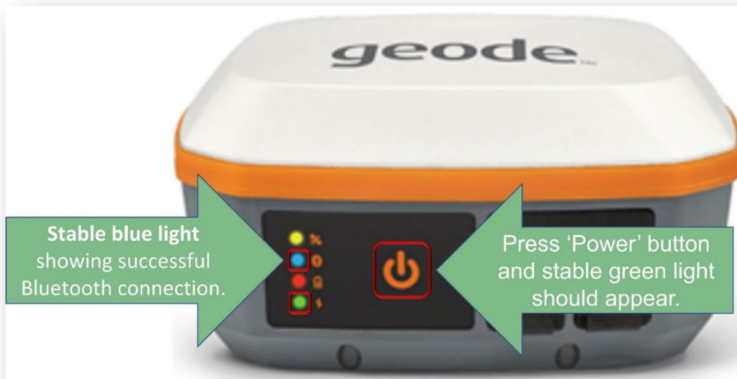
Figure 2.4: Image of the Geode external GPS device powered on and its active connection status. Refer to Appendix 2 for further details on the Geode GPS device.
