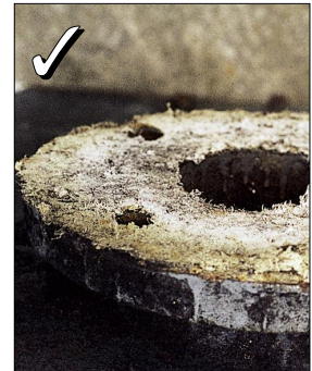
Damaged textured coating, asbestos cement roofing and an asbestos-containing gasket
