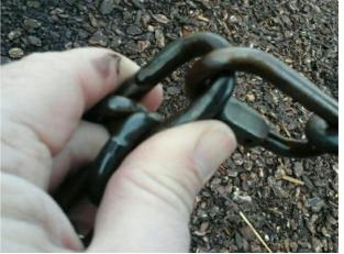
Monitor for any further deterioration and replace when 40% worn
