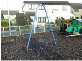
**Finding:** The chain openings are in excess of the 8.6mm as recommended by BS EN 1176
