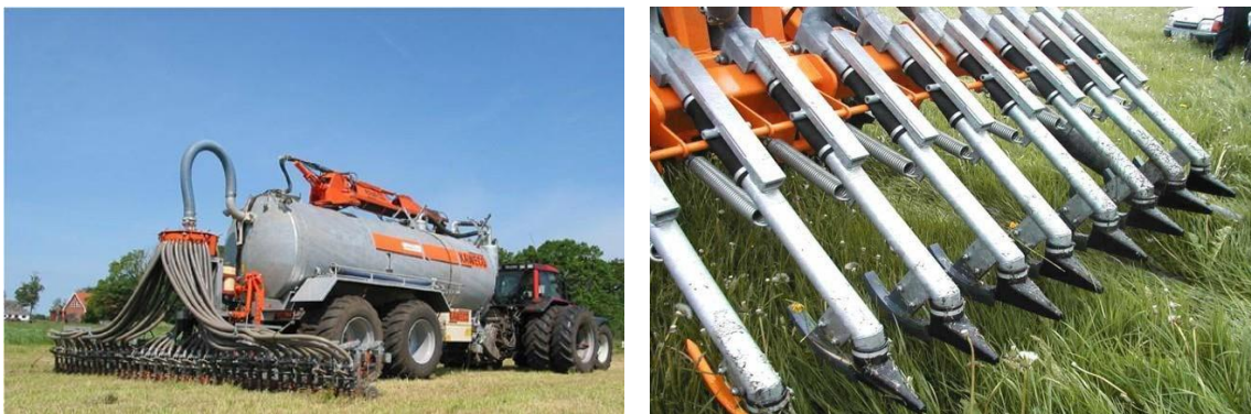
Figure 4. Low emission spreading techniques suitable for grassland: shallow injection (left) and trailing shoe (right) Manure storage
