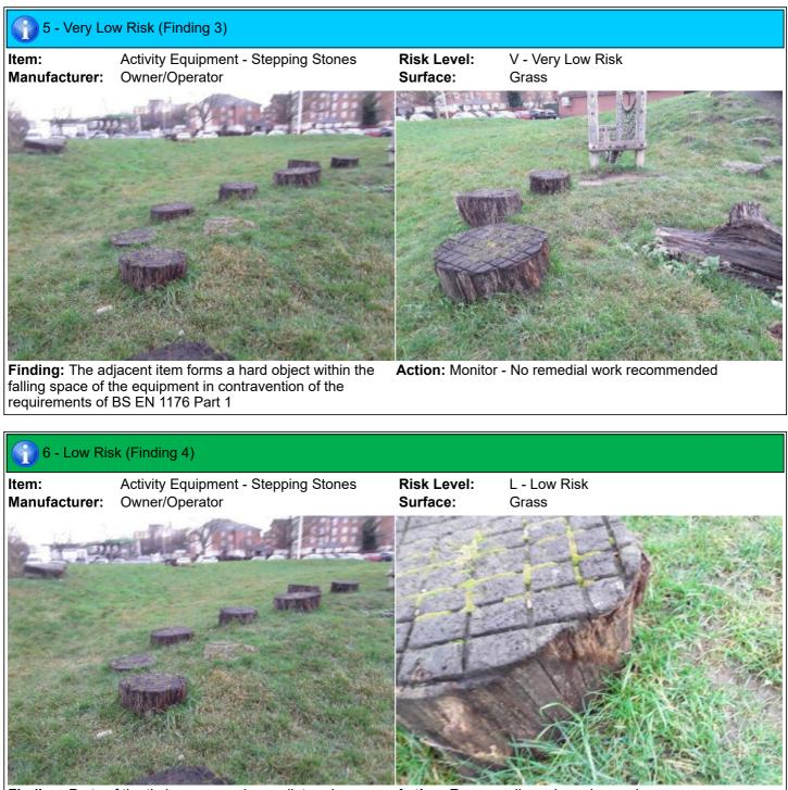
Finding: Parts of the timber are rough or splintered
