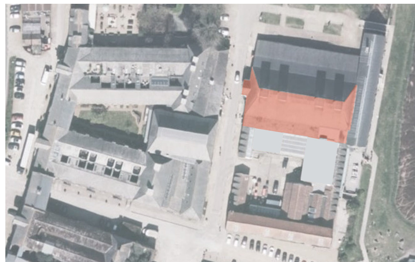
East, South, West roofs and upper flat roof require re-roofing and insulation
