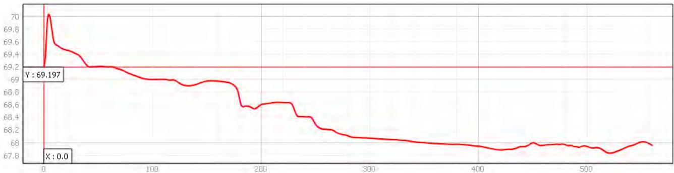
Figure 7 – Option 2 Elevation Profile from Gelvert Stream bed down to the lake (based on Topographic Survey)
