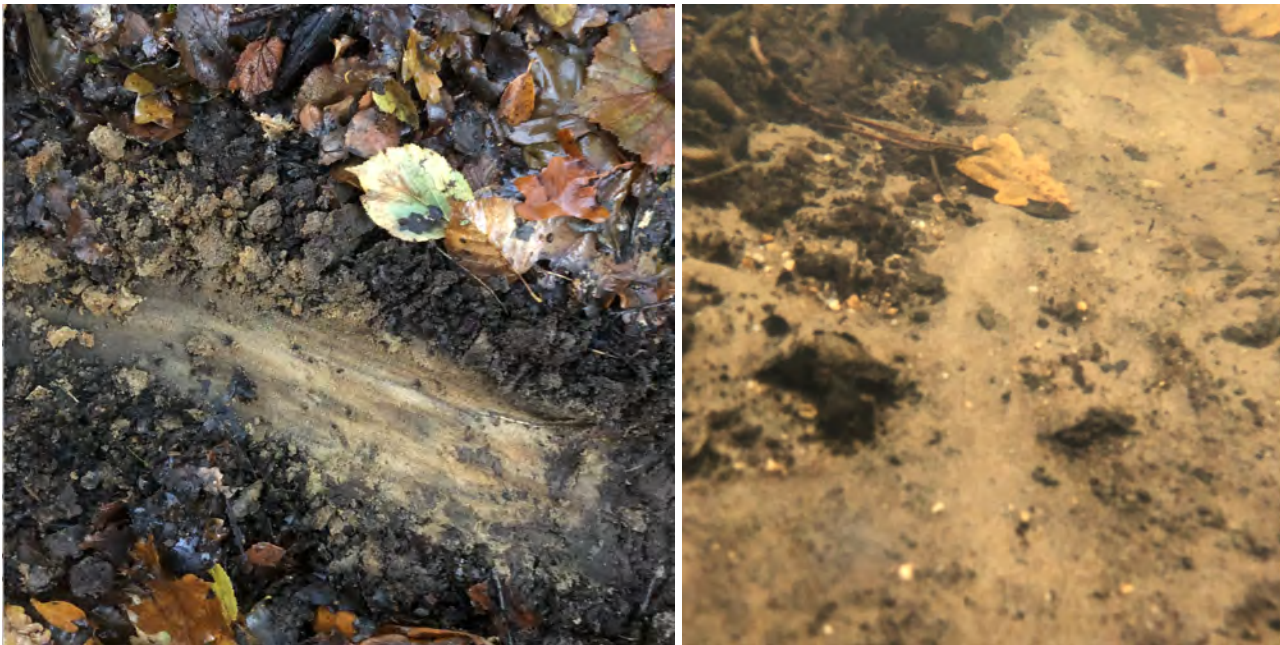
Plates 1 and 2. Sand deposits below leaf litter within the lower diversion link and sand deposits on the bed of the upper diversion link.
