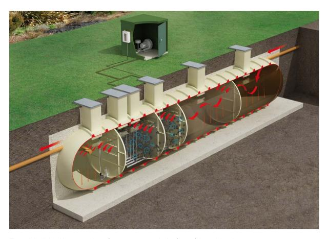
The unit is divided into a number of compartments. At the front of the unit is a large two stage compartment, the purpose of which is to provide a settlement zone for the primary solids. The settled liquid, free from gross
