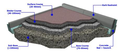
The perimeter of the car park to have kerb edging to be installed as per the design below with associated quadrant and dropper kerbs as required. These are to be bedded /haunched on a 20mm aggregate concrete base proportionate to the subbase/ base layer in the above diagram.
