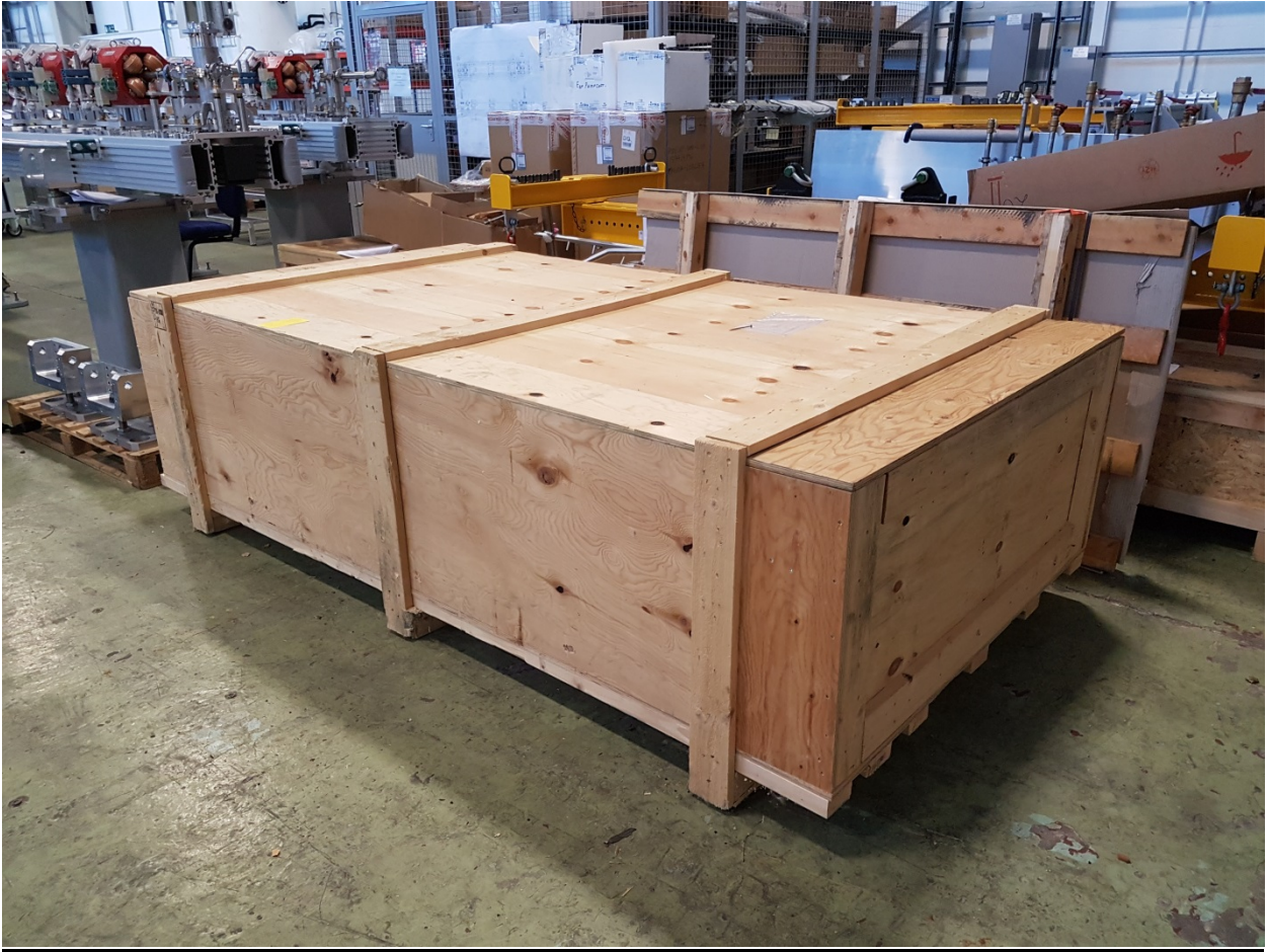
Figure 9: Typical case construction for a fork lift.
