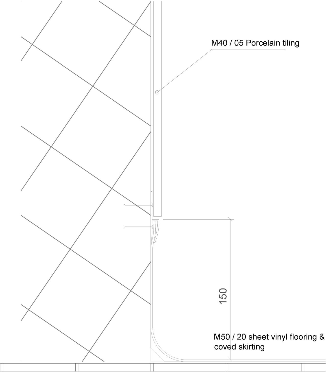
Typical floor skirting detail
