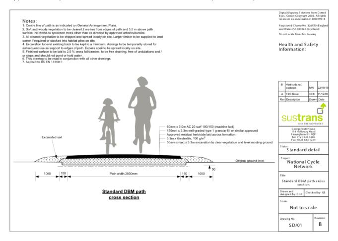
Regrade soil to edges of tarmac on completion using material saved when track excavated.
