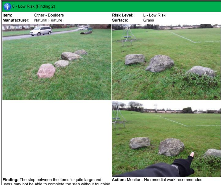
**Finding:** The step between the items is quite large and users may not be able to complete the step without touching ground, the items could therefore be considered to be within the falling space of each other, however the intention of the play activity continuity is easily apparent and foreseeable to the user
