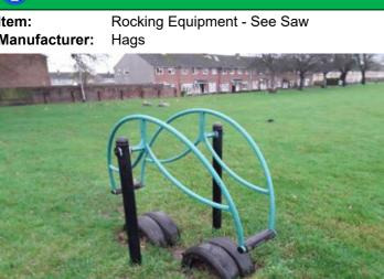
Finding: The rubber foot cover has been damaged
