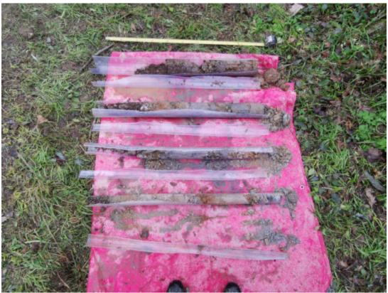
Photograph 6 – Window Sample Hole WS1
