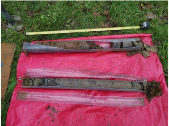
Photograph 5 – Window Sample Hole WS2
