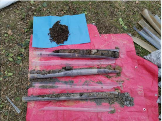
Photograph 3 – Window Sample Hole WS4
