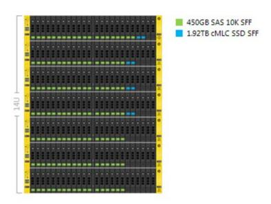
With the addition of the optional components namely 12 x 450GB FC SAS disks. The 3PAR will deliver an additional 3.6TB of usable storage at RAID5 (3+1) and an additional 1083 iops on the SAS Tier.
