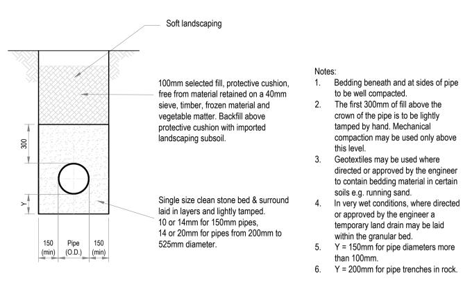
CLASS S BEDDING FOR PIPEWORK WHERE COVER TO SOFFIT IS MORE THAN 600mm BEDDING FACTOR 2.5 Scale 1:20
