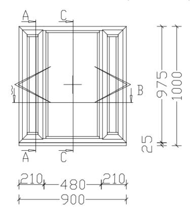
Drawing 2 – Casement Window (fitted with friction stay hinges and locking mechanism)
