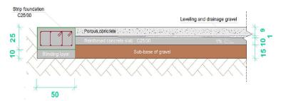
As an alternative you can use a simple reinforced concrete slab with a slope on the short side (10m) of 0.7% -1%
