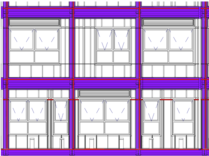
Figure 7: Cavity barrier arrangement in the external wall construction (red indicates the location of cavity barriers)
