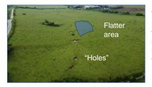
Within the joined runoff pathway, it appears a number of "holes" have been created to store water and slow flow. The flatness analysis suggests a limited area of flatter land which could be connected as a floodplain to raise local water table so it is proposed that the storage features remain.
