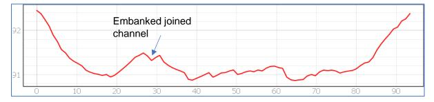
It appears that the current track crossing culvert is not at the lowest point in the natural valley form. Rather than move the culvert, it is proposed to restore the downstream joined flow back into the lower lying land by infill of the embanked channel through pushing the right bank (looking downstream) material into the channel. The combined flow from the culvert should be allowed to spill into the downslope field as a diffuse flow without concentration into any channel.
