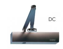
The GEZE TS4000S EN 1-6 / EN 5-7 Door Closer is a heavy duty overhead door closer with a 120 minute fire rating. It is approved for use on doors with leaf widths up to 1400mm (EN 1-6) or 1600mm (EN 5-7). The closing speed and latching action are adjustable and it comes with back check and delayed
