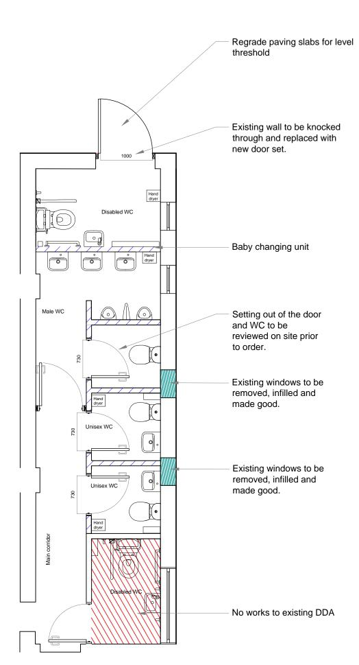
Allow for installation of new stud work walls, comprising 75x75mm studs, 9mm ply, 12.5mm plasterboard, skimmed and decorated both sides. Position to be fixed full height to the
