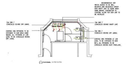
, INSTANTANEOUS HOT WATER HEATER TO BE WALL MOUNTED AND RELOCATED UNDER NEW VANITY UNIT TO SERVE WASH HAND BASINS IN EACH WC. ALLOW FOR NEW UNIT TO BE INSTALLED
