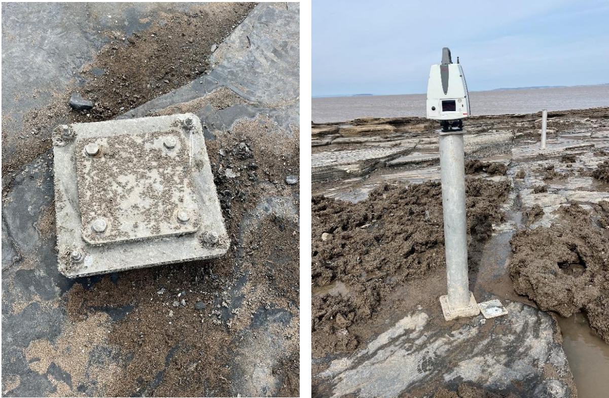
Figure 5: Mounting pole fixed plate with removable protective cover (left) and the Leica P40 Laser scanner on mounting pole (right).
