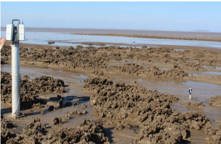
Figure 4: Leica P40 scan station on a mounted pole with a target at the MS site.
