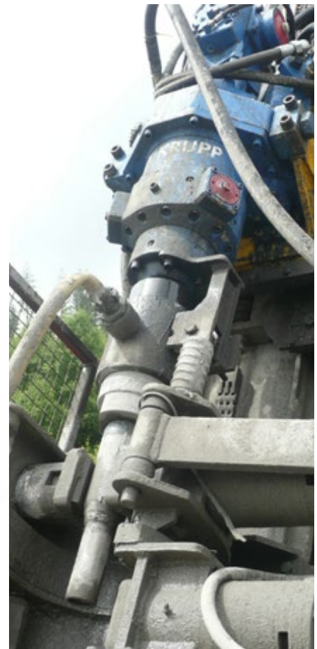
Drill head with simultaneous drill & grout feed
