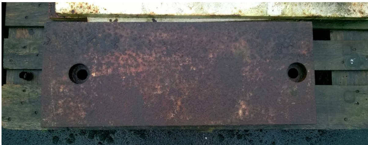
Figure 9. Photo of old counterweight plate.
