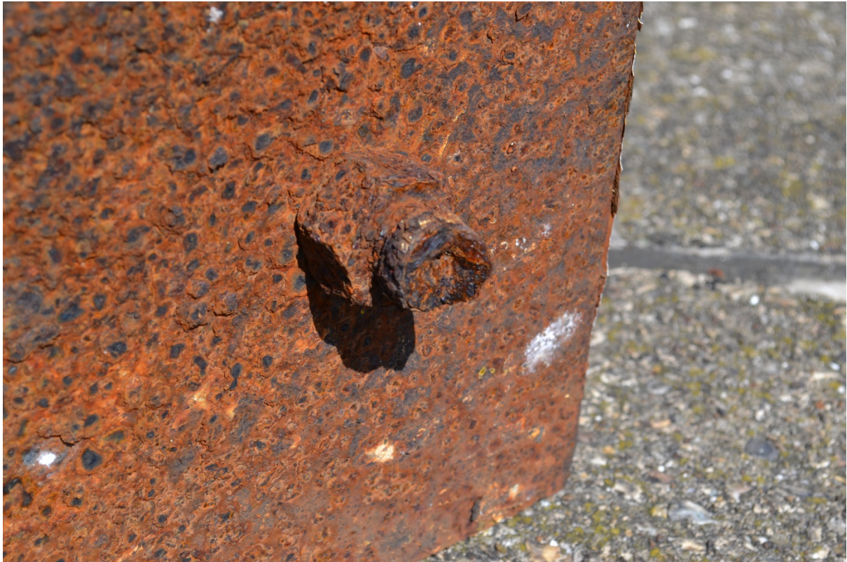
Figure 11. Close-up showing severe corrosion on nut and stud at point where the stud failed.
