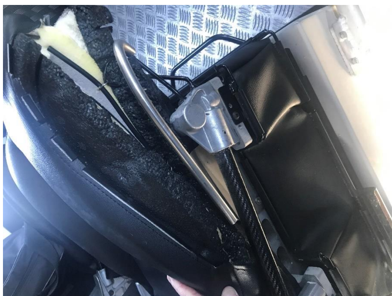
Defect 7 picture. Degraded seat base
