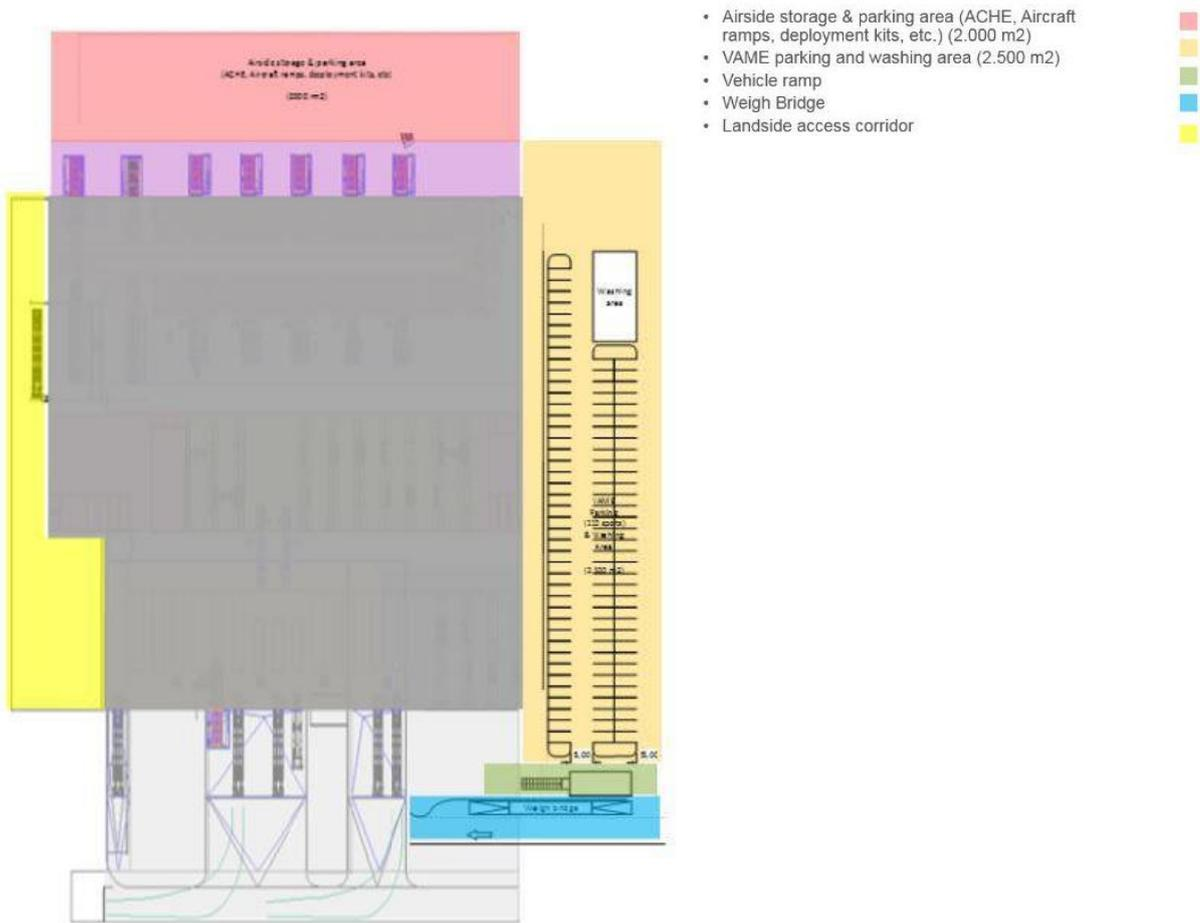
Figure 3: Indicative block plan of external areas
