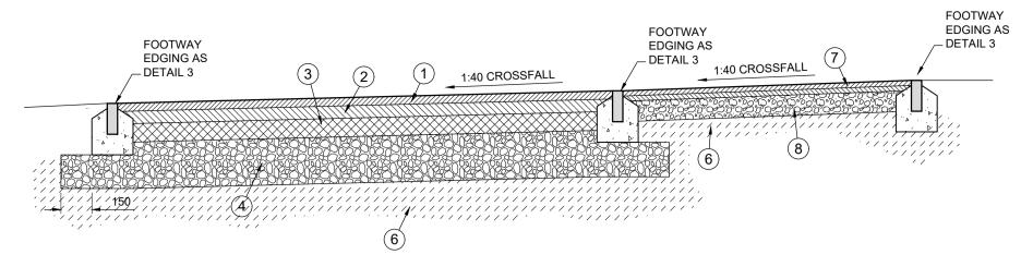
TYPICAL CONSTRUCTION DETAIL FOR ACCESS DRIVE
