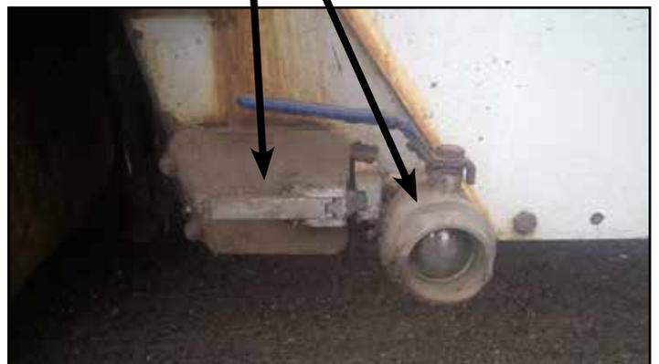
Area at the front of the ejector blade (ie behind cab) – access via locked side-entry door, including drainage pipe clearance to allow liquid run off.
