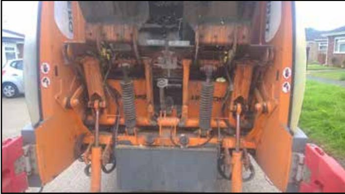
Hopper area including entire rear of sweep blade housing, especially the top of the carrier.
