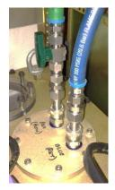
Example of water fitting style used on other equipment (ref <a href="www.swagelok.com/en/catalog">www.swagelok.com/en/catalog</a>) fitting eg SS-600-6
