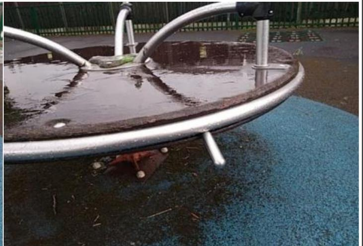
**Finding:** There is/are finger entrapment/s in the underside of the platform and the item fails to meet the requirements of BS EN 1176 Part 1 4.2.7.6 Entrapment of fingers
