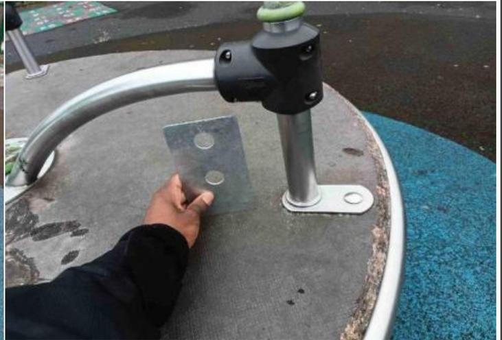
**Finding:** The item fails to meet the requirements of BS EN 1176 Part 1 4.2.7.2 for head and neck entrapment in the handgrip
