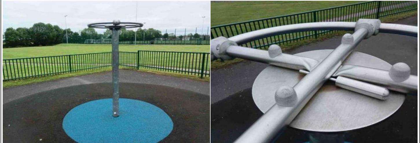
**Finding:** There is/are finger entrapment/s in the handgrip and the item fails to meet the requirements of BS EN 1176 Part 1 4.2.7.6 Entrapment of fingers
