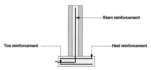
Toe mesh - A393 - (393 mm²/m) Heel mesh - A393 - (393 mm²/m)
