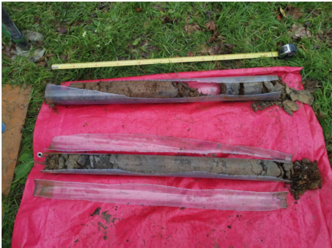
Photograph 5 – Window Sample Hole WS2
