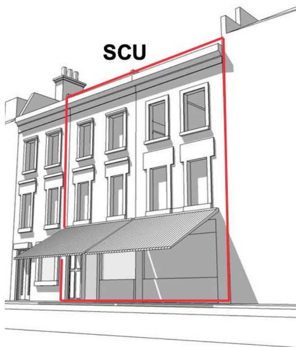
Figure 1 The assignment of a self-contained unit (SCU) around a ground floor shop that spans two buildings (e.g. 7 – 9 The High Street) with domestic flats above. The SCU is designed so that it does not divide any premises and treats the enclosed objects as a single unit.
