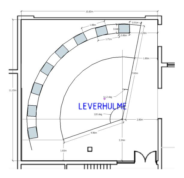
The following diagram shows the approximate dimensions measured from the current display system and shown in a potentially viable position in the designated room in Building 2 in the new Hartree Centre Visualisation facility
