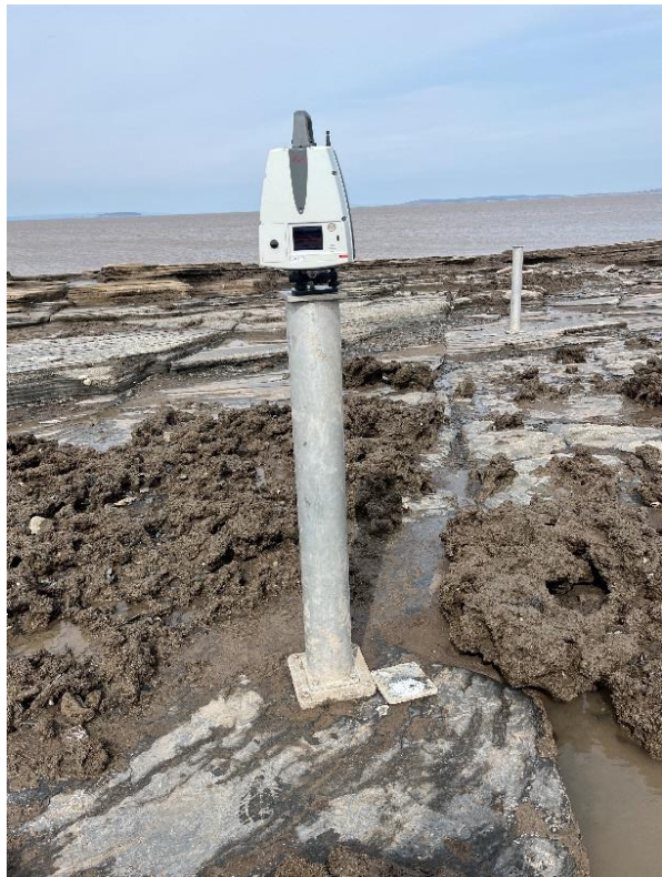
Figure 6: Mounting pole fixed plate with removable protective cover (left) and the Leica P40 Laser scanner on mounting pole (right).
