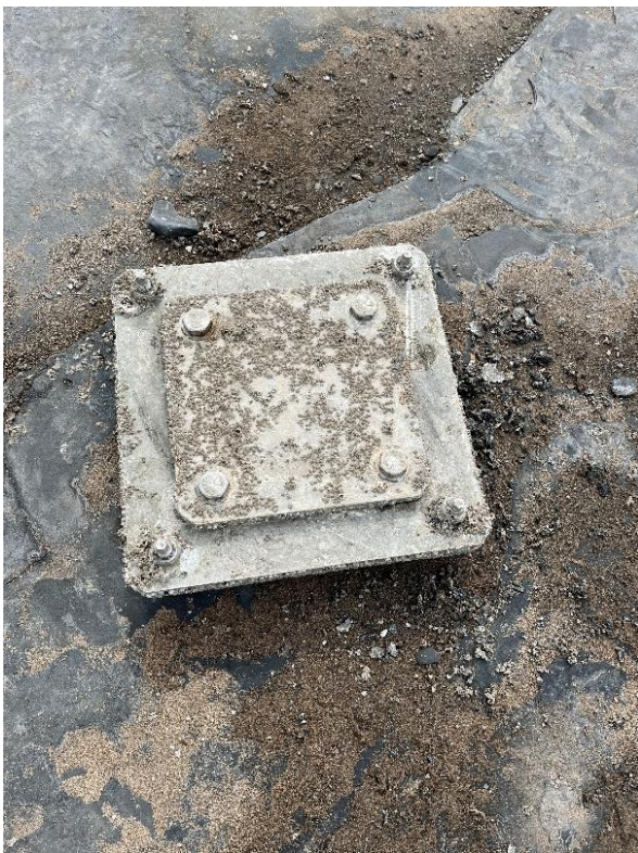
Figure 6: Mounting pole fixed plate with removable protective cover (left) and the Leica P40 Laser scanner on mounting pole (right).
