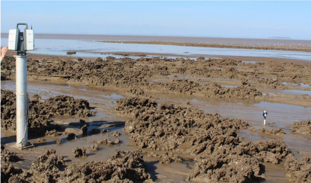
Figure 5: Leica P40 scan station on a mounted pole with a target at the MS site.
