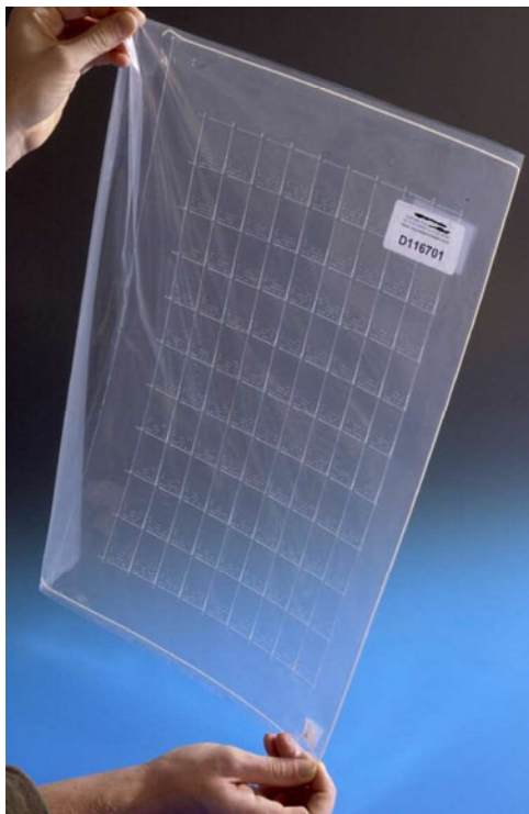
Fig. 1. Cut and encoded PADC sheet in polythene bag
