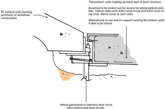
Bearing shoe to head of screw pile to
