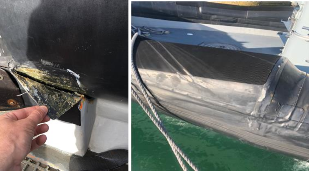
Defect picture 2. Sponson detachment / wear.
