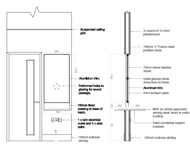
**Note:** This drawing is only to be used for understanding the construction and size of the reception counter and screen being proposed. The wall and door construction are not applicable to this scheme.
