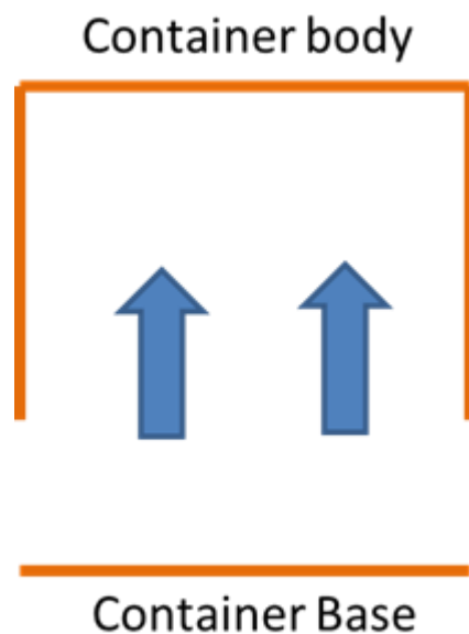
Figure 3-1: "Top-hat" container body which lifts off of container base.
